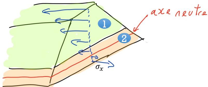
$$N = 0 = \iint_{\text{section1}} \sigma_{x1} dA + \iint_{\text{section2}} \sigma_{x2} dA$$
